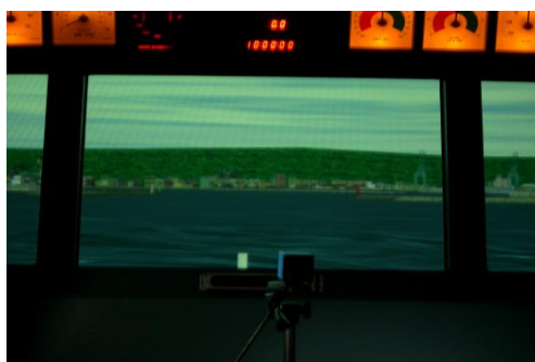
Fig. 4 the CCD equipment arrangement in the simulator bridge
